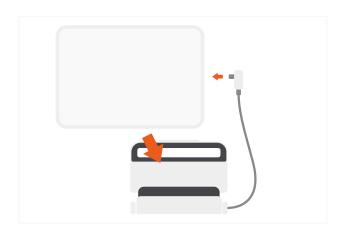
3 Use the HDMI port to output 4K display to compatible HDMI-enabled monitor – up to 60Hz. Requires a direct HDMI connection
